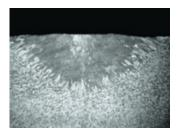
VARIGON He50. Shielding gas for TIG and MIG welding of slightly coarser aluminium. Increased metal penetration and flow with the addition of helium. Enables a higher welding speed.
