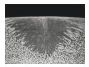
VARIGON He70. Shielding gas for TIG and MIG welding of primarily coarse aluminium. Increased metal penetration and flow with the addition of helium. Enables a higher welding speed.
