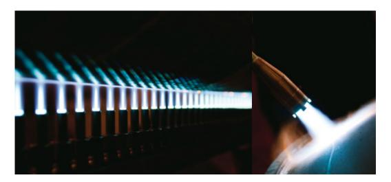
LINDOFLAMM® is a complete system for heating of large work pieces, flame straightening of thick plates, sealing of flame sprayed coatings and hot forming of thick plates, tubes and profiles.
