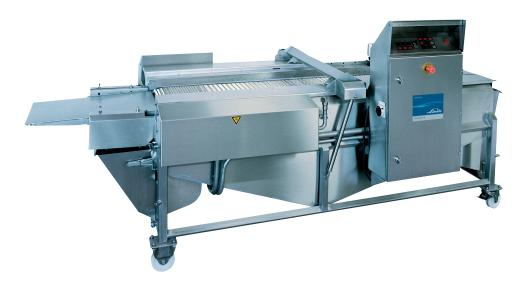
If you are looking for ways of producing frozen pellets of sauces, purees and other liquid foodstuffs, then take a closer look at the CRYOLINE® PE. This patented freezer will produce IQF pellets in a regular size with high repeatability, opening up many possibilities for the modern food processor. If you are producing for the catering or retail market, this freezer will allow your customer to defrost as much or as little of your product as required, giving you the edge over your competitors.
